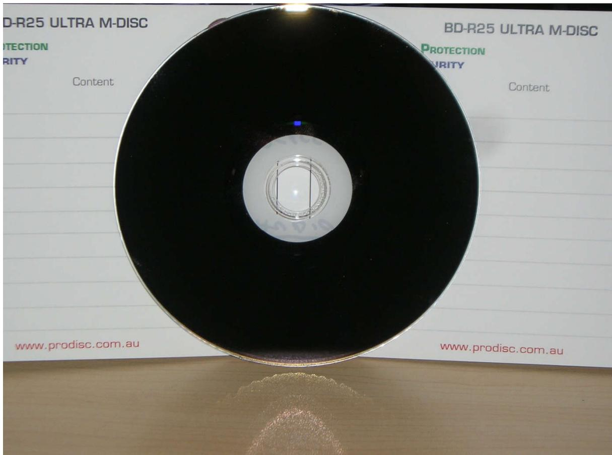
Unlike other recordable optical media, the **PRODISC Ultra M-Disc** does not use an organic dye layer to store the data. Instead it uses a special carbon compound (referred to as the “Stone Recording Layer”) into which the Blu-Ray laser “engraves” the information thus eliminating the possibility of long term dye rot leading to permanent loss of information.
